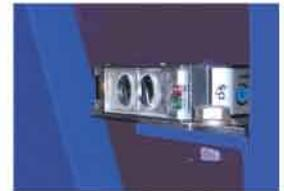
**Oscillating air jet blowers** (optional) for an efficient cleaning of sanding belts, they activate only when the workpiece is being processed.
