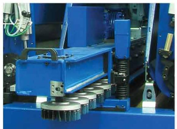
The XVS unit is designed to operate with standard, low-cost, brush cups as well as more specialized, custom-made, brushes.
