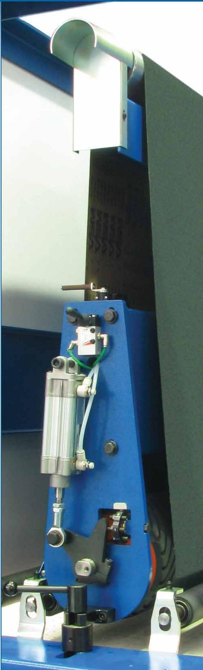
The perimetral deburring unit is composed of an identification system of the geometrical shape of the workpiece to be deburred. It is controlled by a PLC which activates a series of pneumatic sections (with 32 mm or 16 mm definition) that apply the necessary pressure on the abrasive belt on the perimeter of the workpiece only, thus removing the burrs. The advanced system management via PLC allows to vary the amplitude and the pressure of the working area as required.
