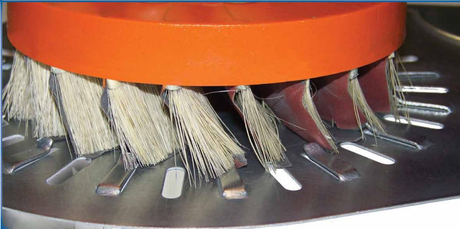
This unit is composed of a series vertical brushes, rotating at high speed (inverter controlled) and oscillating side-ways at adjustable rate of oscillation. Combining the vertical axis rotation with high frequency oscillation allows to achieve a perfect deburring in all directions with a single working unit.
