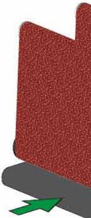
rounding of oxy and plasma cut parts, using a machine in configuration "CCR"
