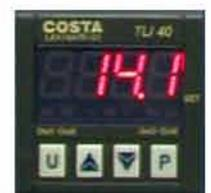
Digital positioner with read-out of the thickness adjustment with decimal accuracy.
