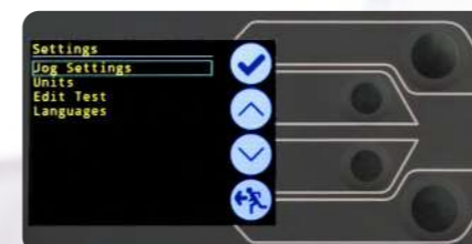
▲ Four multifunction buttons for all settings and operation. Multi-language display.
