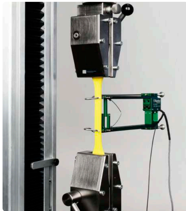
▲ Short-travel axial extensometer
