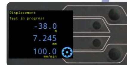
▲ Colour display of speed, displacement and load
