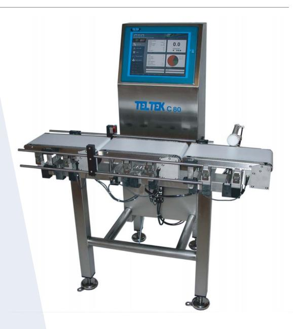
Teltek C80 is a PC based windows XP in line checkweigher featuring a high specification 15" touch screen display for ease of use and maximum operator flexibility.
