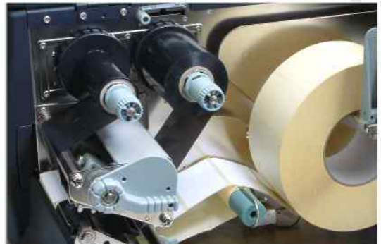
Printer unit with standard Thermal Transfer (TTF) stationary
