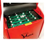
Low rear lift off or roll off for fast changeovers. Good access for battery topping. No motors underneath.
