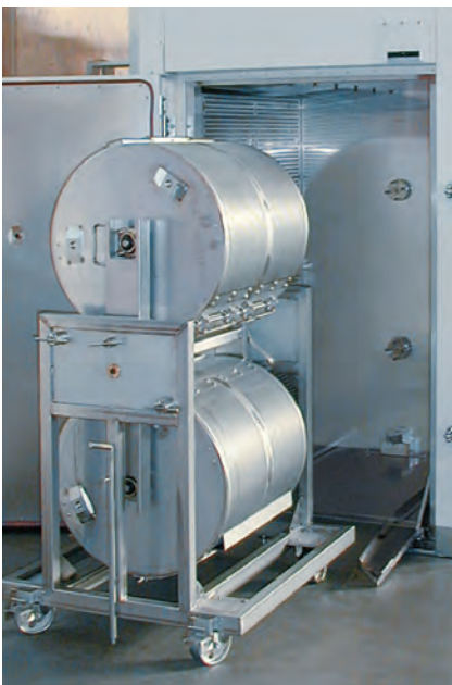
Heat and drying ovens with rotating drum trolley for tempering of small parts/bulk goods
