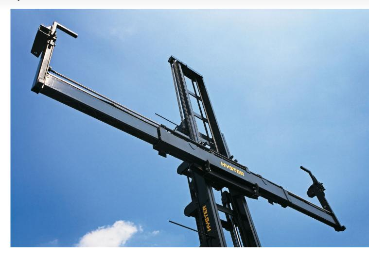
Hyster ECH side-lift 20'-40' telescopic **spreader characteristics:**
