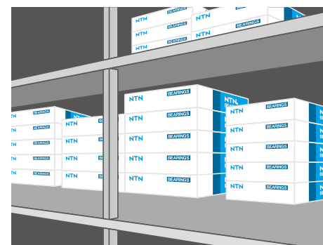
Fig. 15.4 Storing one-bearing boxes on a shelf
