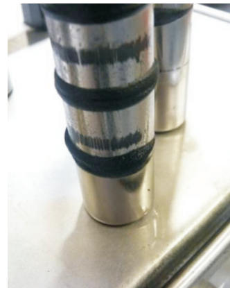
Finest debris collected on magnetic filter rod
