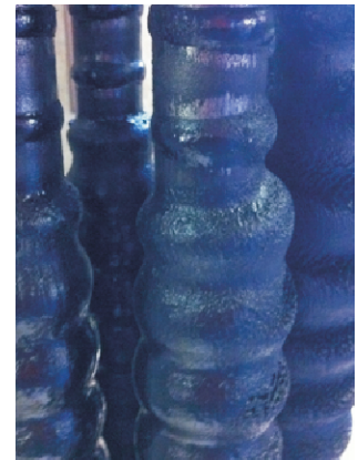
Ferritic particles on magnetic filter rods
