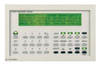
The UPC controller is a 3-Phase AC arbitrary waveform generator and precision AC metering system. Each waveform stored in the UPC is encoded with 12-bit amplitude and 10-bit time resolution for each cycle. The waveform for each phase may be independently selected and varied in amplitude and phase angle with respect
