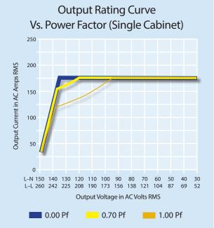
Rated continuous load current as a function of Power Factor and Output Voltage–Nominal Input Line.
