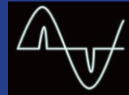
Programmable Output Impedance Same conditions as above with programmable Z 0 engaged. THD=0.25%
