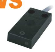
The acoustic sensor detects defined static noise or switch-sounds on machines, devices and plants. Due to protection class IP67, an enlarged operating temperature up to 85°C and an adjustable switching threshold this sensor even is proper for external applications.
