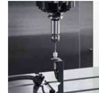
Tool breakage detector, touch type A touch switch type tool breakage detector is available.
