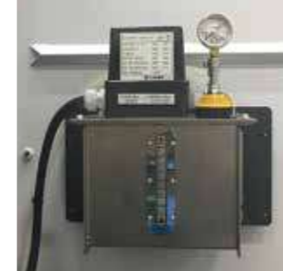
Automatic oil lubricator Regularly applies oil to all lubricating points on the tree axes.
