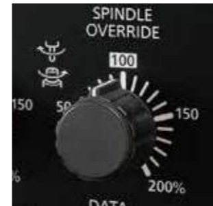
Spindle override Spindle speed can be changed without changing the program.
