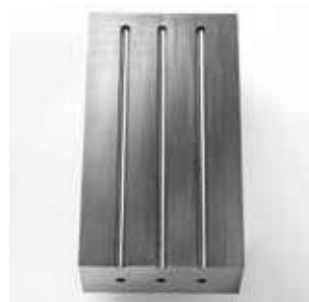
ø6 × 170mm (L/D=28) Workpiece: Carbon steel
