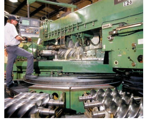
CycloBlower XP rotors are precision ground using state of the art milling technology.
