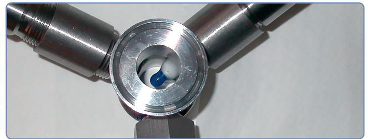
Figure 2: DO sensor (left), pH sensor (right) and sample port (in front) mounted between static mixer modules of the PFR
