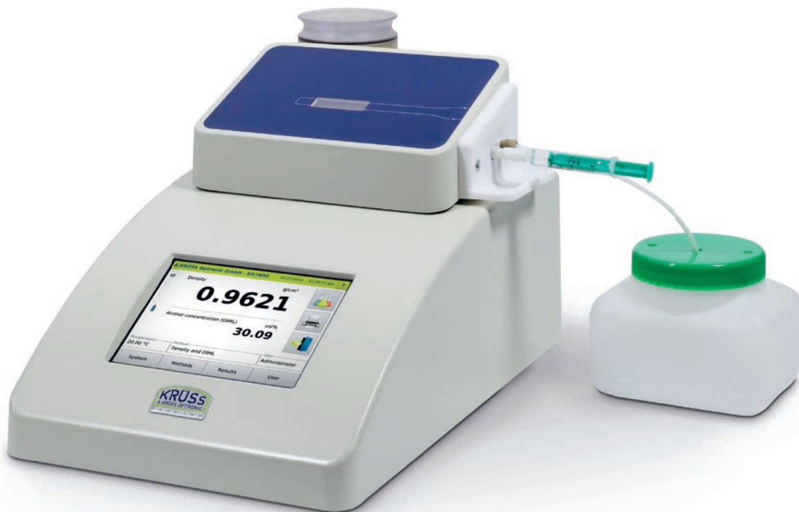
Manual sample supply via syringe
