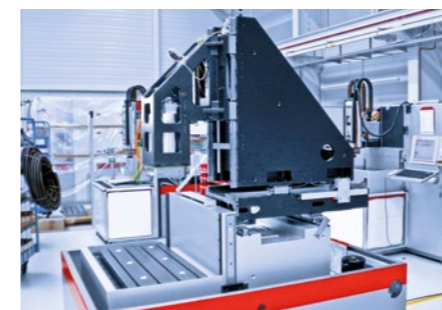
X-Y-slides Guaranteed accuracy through oversized slides and guides.
