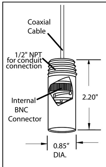
**CPVC and KYNAR CABLES EXPOSED CABLE CONNECTION (NO ATC) - S648, S648K**
