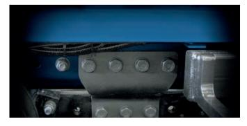
**Fast installation** The hooklift is quickly and reliably bolted on the frame.
