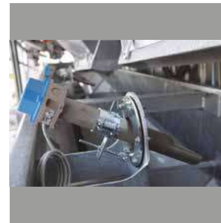
Microwave or resistive aggregates moisture probes. Sonde umidità sabbie a microonde o resistive.
