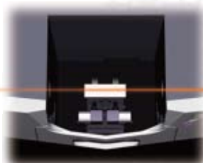
Flame measurement: Burner head intersects the light axis (red line).
