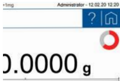
PT: Real-time stability Indicator with visual stability prediction
