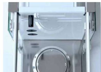
AOS - Ambient observation system records various ambient air conditions what can affect your weighing result. Or shall the balance correct the weighing results with the app BEST?
