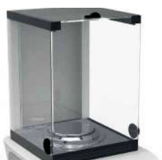
321 LX: Ergonomically designed draft shield
