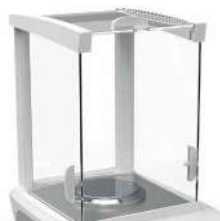
321 LG: Well-tried all-round basic draft shield
