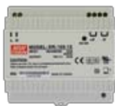
PS100D Power Supply (In: 110/220Vac, Out: 15Vdc/6.5A)
