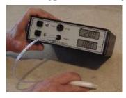
The Quantek Model 907 is a highly portable oxygen and CO2 analyzer used for the measurement of oxygen and carbon dioxide in gas-flushed (CAP/MAP) food packages and process applications (such as sampling chambers).
