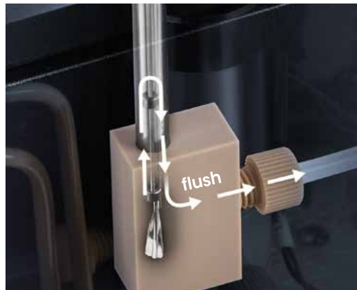
Dedicated Wash Station
