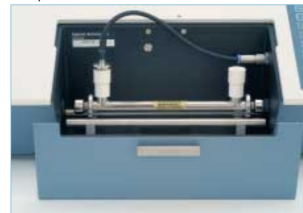
Single sample tube in-situ with dip-in temperature sensor
