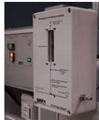
HT/HP inlet (up to 30 bar at 200°C)
