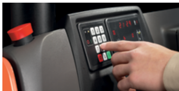
Unique to BT, Reflex M offers PIN-code entry as standard to ensure that the truck is only used by authorised personnel
