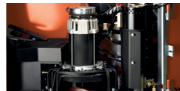
The absence of carbon brushes and power contacts in its AC drive motor reduces maintenance downtime
