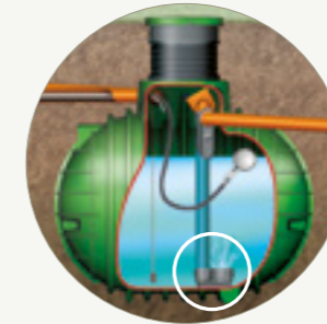
Cleaning stage 2 Steady inflow The finest dirt particles settle at the bottom of the tank as sediment. The filtered water is introduced through an inlet pot in the tank base. This permanently prevents the sediment being stirred up.
