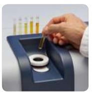
Open sampling positions at all measurement channels with no need to open covers or drawers.
