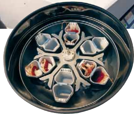
Image showing the rotor and double buckets for quad and triple blood bags of 500 and 800 ml.
