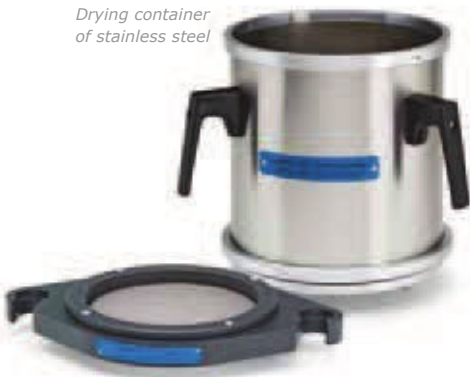
Clamping cover with replaceable filter fleece insert
