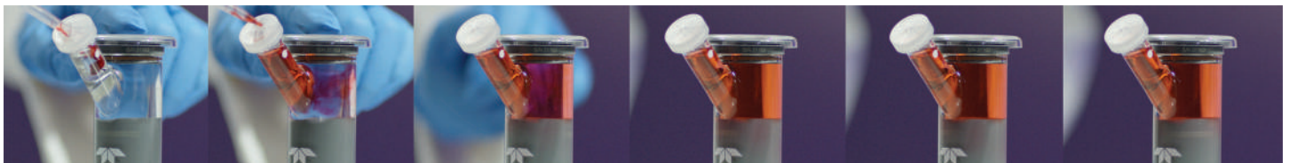
Visual testing of mixing effectiveness by dispersion of red dye placed on top of media in the sampling arm with images at 1 second intervals from 0 to 5 seconds while mixing at 400 rpm.
