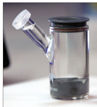
Meniscus through center of fill mark conveniently indicates receptor media has reached the level of the membrane.
