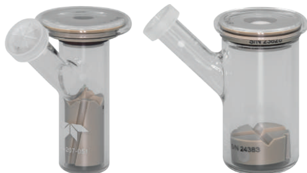
Small cell with tall mixer-insert provides 10 mL receptor media volume.
