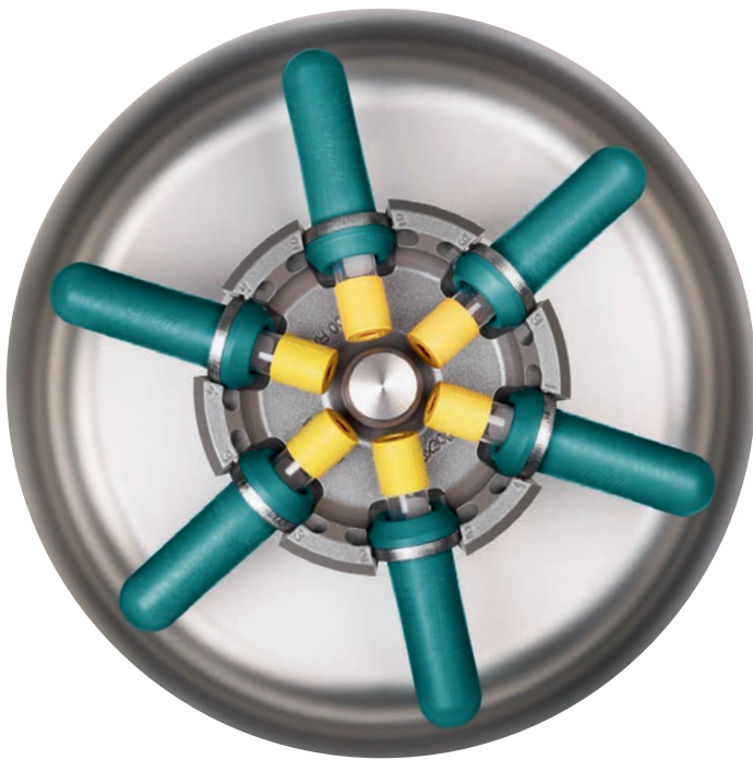
View into the centrifuging chamber showing the rotor 1146 with blood collection tubes
