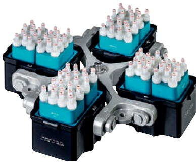
illustrated with carriers 5628, adapting frame 5220-A and adapters 5258
