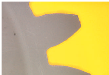
Plastic Gear Teeth with Smaller Module
