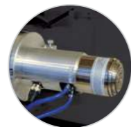
180 kV TRANSMISSION TARGET
