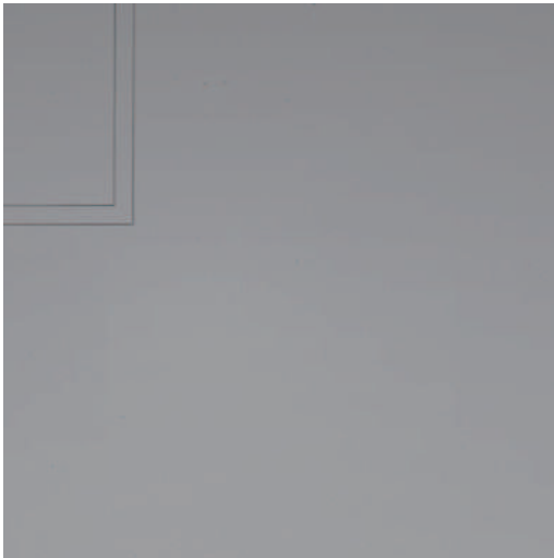
Laser Image without DIC (5x Objective) STEP Height standard Type B, PTB-5, Institut für Mikroelektronik, Germany
