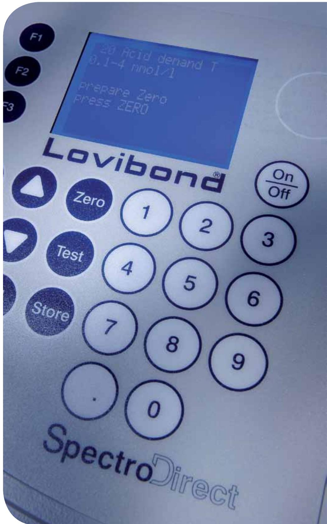
The SpectroDirect is a modern single-beam spectrophotometer with an excellent price/performance ratio that is specifically designed for water testing.
