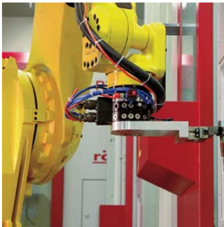
Robot loading of tool changer
