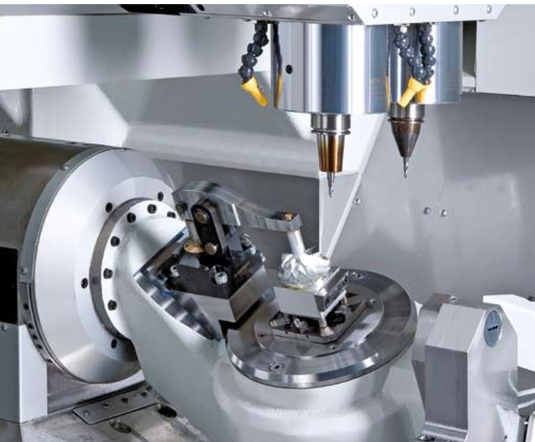
Machining area of the RXS 500 DSI2, set up for impeller machining
